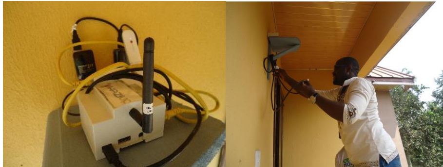
Figure 2: Deployed gateway in the office of Kumah Farms, 300m far away from the device
